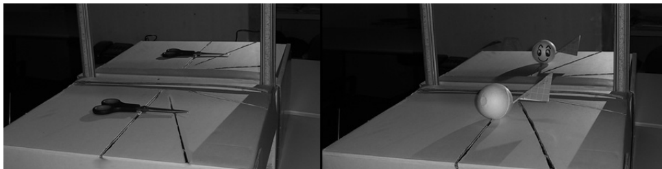
Figure 5.3 A pair of scissors (on the left) and a puppet (on the right) in front of a plane mirror. The reflection of the pair of scissor is perceived as having an identical orientation to the real object, while the reflection of the puppet as having an opposite orientation.
